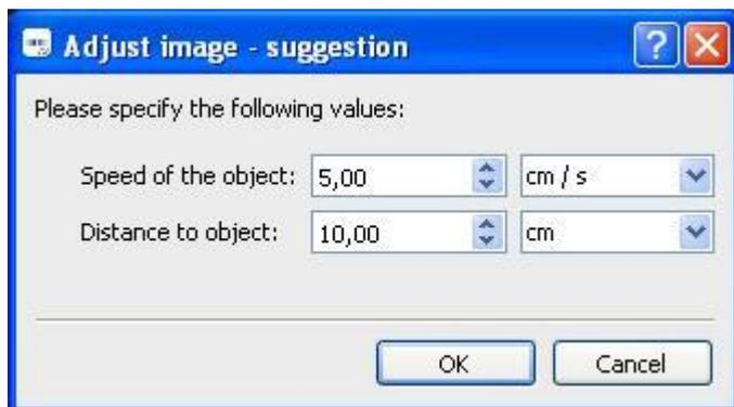
Enter the speed of the objects, and their distance from the camera, during inspection. The *Application Suite* automatically calculates the associated parameters. If the image is then still too dark or bright, you can adjust this using the control gain (Amplification).
