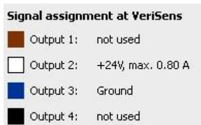
This view shows how the signals at the 4 outputs of the illumination port are connected for the current settings.
