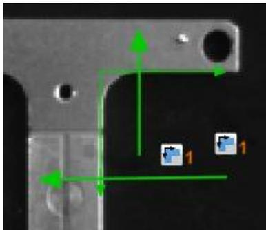
In this example, two edges of a test object are found, with a horizontal and a vertical search line, and the reference point for part location is determined at the intersection of the detected edges.
