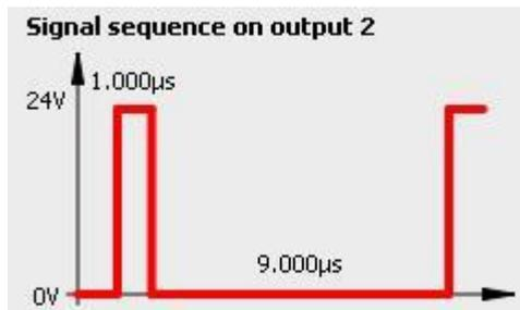
This diagram shows the current waveform at output 1 and output 2.
