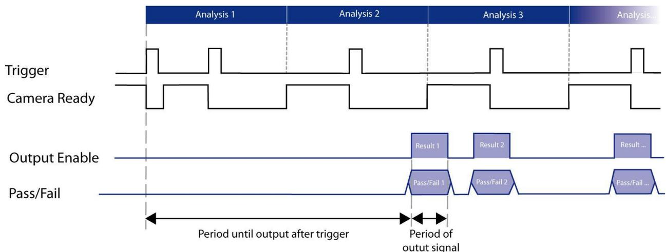
Following image acquisition, the *Camera Ready* signal is deactivated. The *Camera Ready* signal is activated again at the end of image acquisition and another image acquisition operation is possible immediately.
